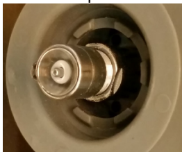
Figure 2. Priming Lixit for Weanling Cages. Lixits should be primed at the time of weaning. For new weanlings, prime lixit more frequently. (Note: If a Lixit drips continuously, immediately remove cage from the Lixit to prevent flooding, and notify LARC.)
